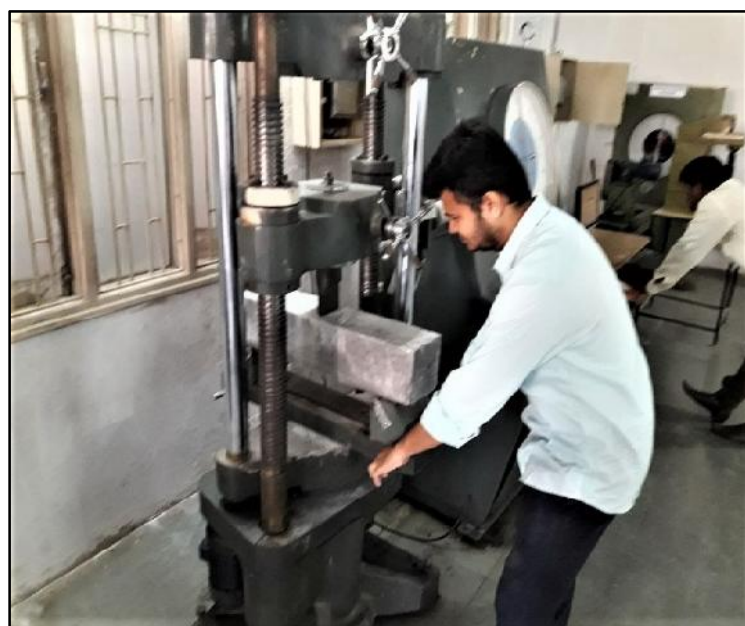
Fig.7: Performing Flexural Strength Test on Beam
