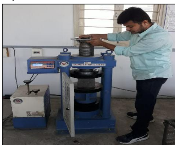
Fig.1: Performing Compression Test on Cub
