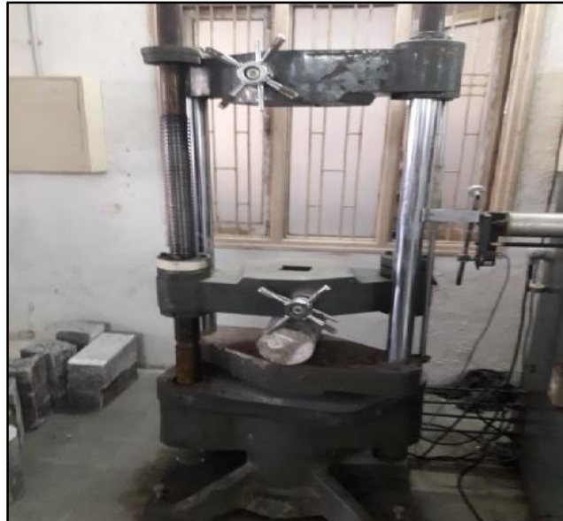
Fig.4: Performing Splitting Tensile Strength Test on Cylinder
