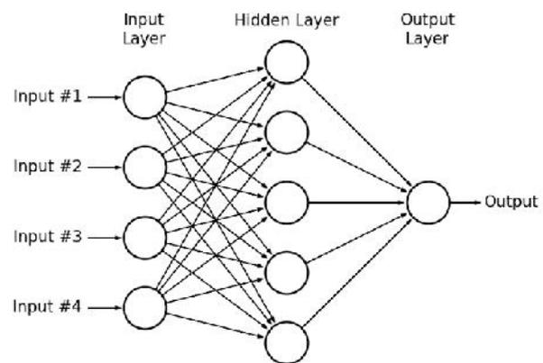
FIGURE 2. LAYOUT OF INPUT OUTPUT IN ANN
