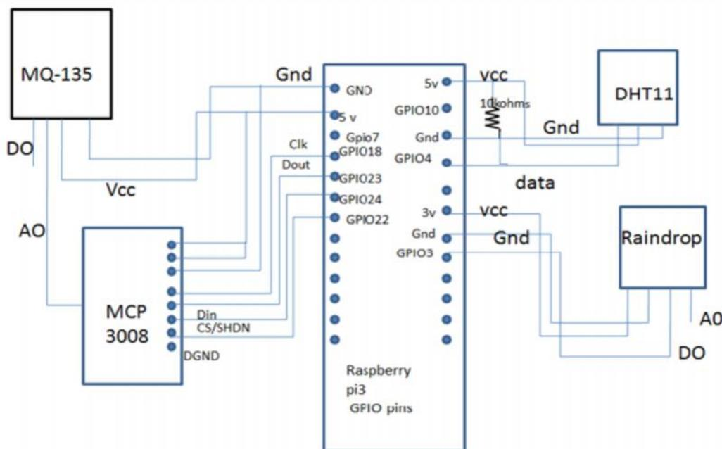
Fig 1: Proposed system architecture of a node.
