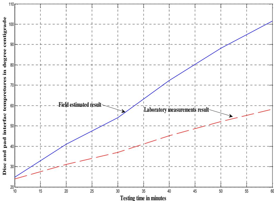
Figure 5.1 shows the results obtained using the developed test rig and estimated field readings for better
