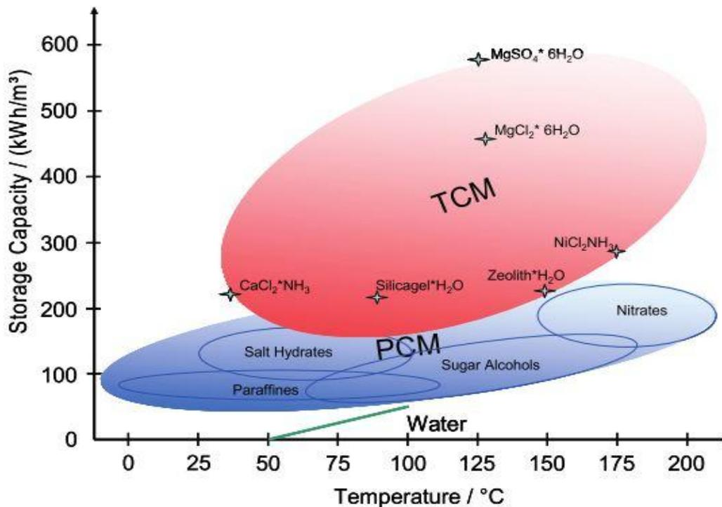
Fig. 2: The comparative of storage capacities of sensible, latent and thermochemical heat storages.
