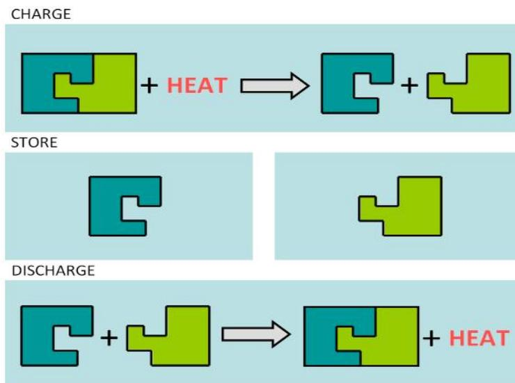
Fig.1: Working principle of Sorption Thermo Chemical TES system
