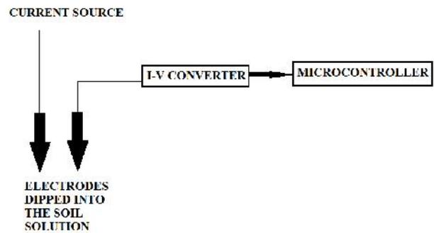
Fig: 6 Electrical conductivity measurement
