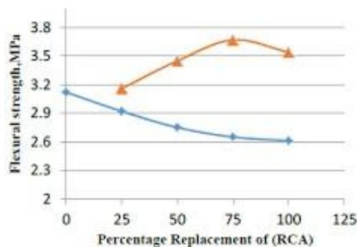
Variation of flexural strength at different replacement level
