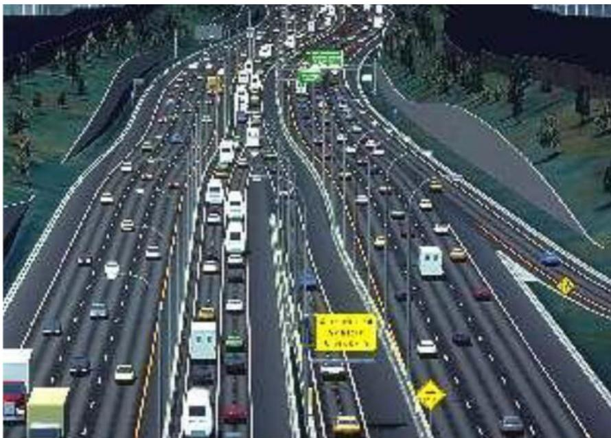
Figure 2.1 – A concept drawing of an Automated Highway System with dedicated lanes in the centre of the highway.
