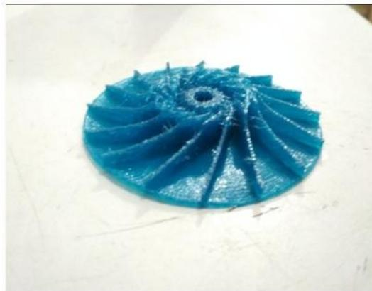
Fig.6.4. Successfully printed part without any defect
