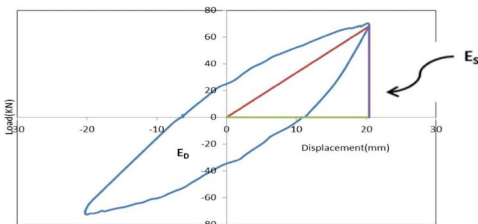
**Fig.** Description of hysteresis and strain energy
