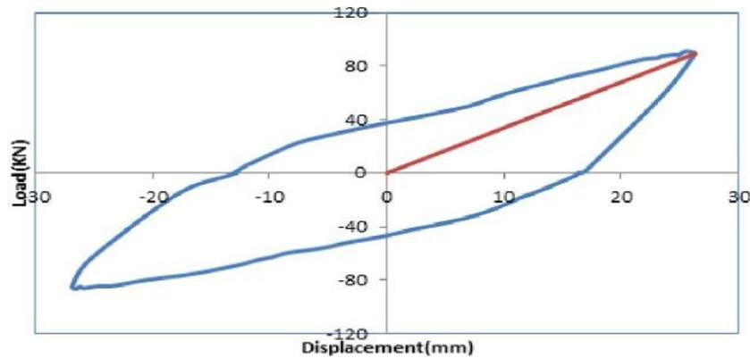
**Fig.** Description of loading secant stiffness
