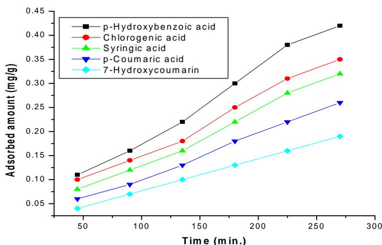
**Fig 5: Adsorption isotherm of phenolic acids onto ACCP at different contact time (pH =6.5, temp. =  $25\pm 0.5^\circ\text{C}$ , mesh size = 100, concentration=10mg/L, adsorbent dosage = 1g/100ml).**
