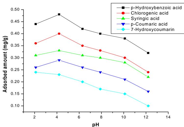
**Fig 7: Adsorption isotherm of phenolic acids onto ACCP at different pH values (temp. =  $25 \pm 0.5^\circ\text{C}$ , shacking time = 5h (200 rpm), mesh size = 100, adsorbent dosage = 1 g/100 ml).**
