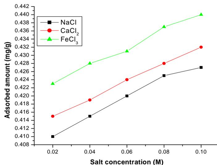
**Fig 10: Influence of ionic strength (cations) on adsorption of p- hydroxybenzoic acid onto ACCP (pH = 6.5, temp. = 25±0.5°C, shaking time = 5h (200 rpm), mesh size = 100)**
