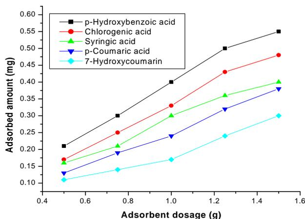
**Fig 6: Adsorption of phenolic acids onto ACCP at different adsorbent dosage (pH = 6.5, temp. =  $25 \pm 0.5^\circ\text{C}$ , shacking time = 5h (200 rpm), mesh size = 100, concentration = 10mg/L).**
