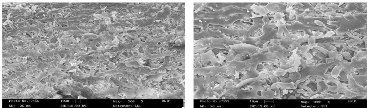
**Fig 3: SEM pictures of activated corncobs powder (ACCP) at 500X and 1000X.**
