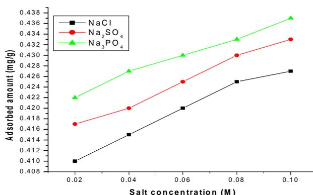
**Fig 9: Influence of ionic strength (anions) on adsorption of p- hydroxybenzoic acid onto ACCP (pH = 6.5, temp. = 25±0.5°C, shaking time = 5h, mesh size = 100)**
