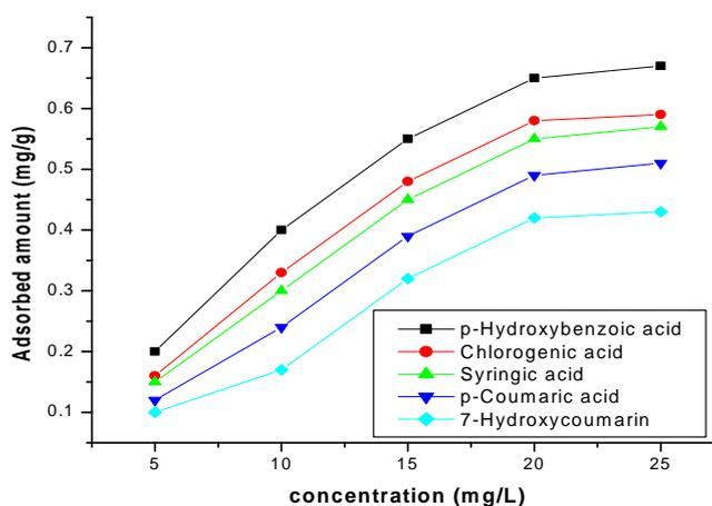
**Fig 4: Adsorption isotherm of phenolic acids onto ACCP at different concentration (pH= 6.5, temp. =  $25\pm 0.5^\circ\text{C}$ , shaking time = 5h (200 rpm), mesh size = 100, dosage = 1 g/100 ml.**
