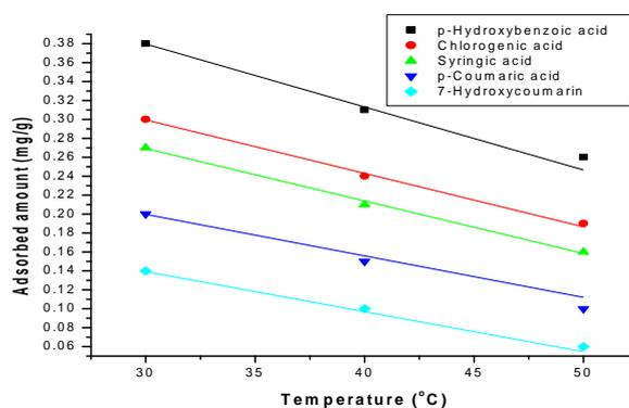
**Fig 8: Adsorption isotherm of phenolic acids onto ACCP at different temperature (pH = 6.5, shaking time = 5h, mesh size = 100, dosage = 1 g/100 ml, concentration = 10mg/L).**
