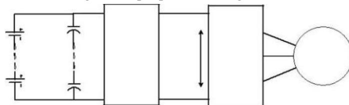
Fig. 3. Passive configuration with DC-DC converter
