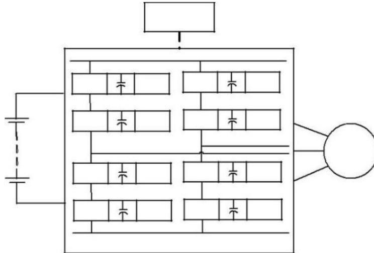
Fig. eight. Modular multilevel configuration
