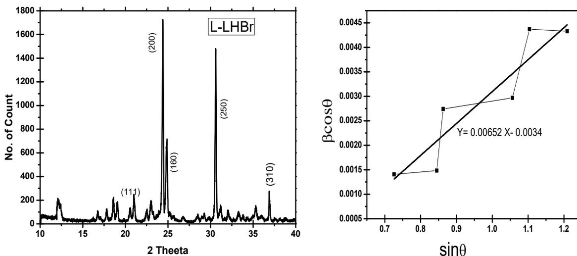
Using the data obtained from powder XRD analysis a curve is plotted between  $\sin \theta$  and  $\beta \cos \theta$  known as W-H plot. From the W-H plot, value of mechanical strain present in the crystal were calculated and found equal to  $+ 1.37 \times 10^{-3}$ . Hence, the positive value of mechanical strength present in the crystal indicates that point defects are present in the grown crystal.
