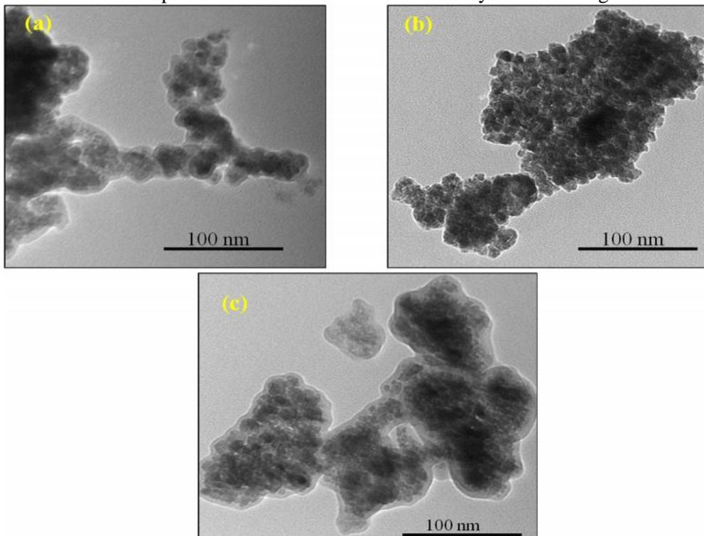
**Fig.5:** TEM micrographs of  $Ni_xCu_{1-x}Fe_2O_4$  (a)  $x=0.2$ , (b)  $x=0.4$  and (c)  $x=0.6$
