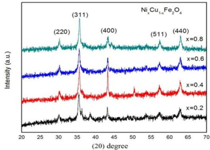
**Fig.1: X-ray diffraction pattern of Ni<sub>x</sub>Cu<sub>1-x</sub>Fe<sub>2</sub>O<sub>4</sub> (x=0.2, 0.4, 0.6, 0.8) samples.**
