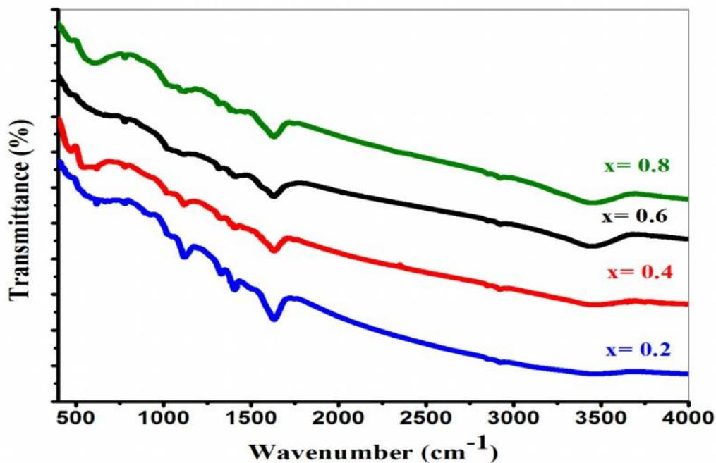
Fig.3: FTIR spectra of  $Ni_xCu_{1-x}Fe_2O_4$  ( $x=0.2, 0.4, 0.6, 0.8$ ) ferrite samples
