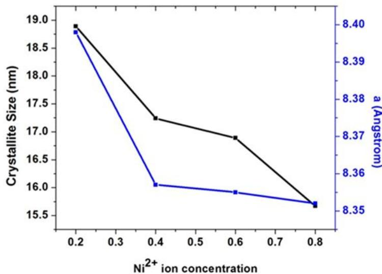
**Fig.2: Variation of crystallite size and lattice parameter with  $Ni^{2+}$  concentration**
