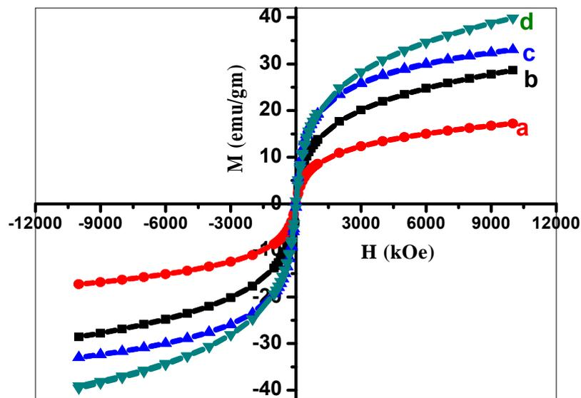
**Fig.6: Hysteresis loops of  $Ni_xCu_{1-x}Fe_2O_4$  samples at (a)  $x=0.2$ , (b)  $x=0.4$ , (c)  $x=0.6$  and (d)  $x=0.8$**
