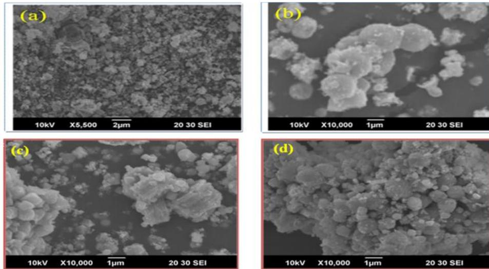
**Fig.4:** SEM micrographs of  $Ni_xCu_{1-x}Fe_2O_4$  (a)  $x=0.2$ , (b)  $x=0.4$ , (c)  $x=0.6$  and (d)  $x=0.8$  samples
