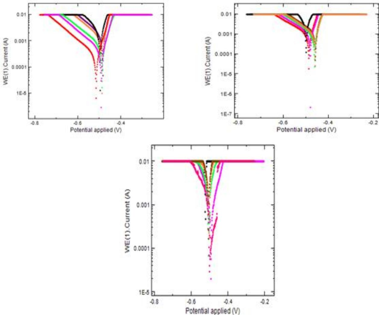
Fig 2. Potentiodynamic polarization curves for low alloy steel in  $H_3PO_4$  in the presence of Calotropis procera with concentration from 100 ppm to 1000ppm.
