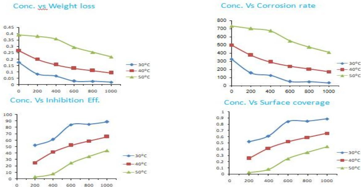
**Fig 1.**Graphical representation of weight loss, corrosion rate (CR), surface coverage ( ) and percentage inhibition efficiency (% IE) with various concentration of Calotropis procera inhibitor at different temperatures.
