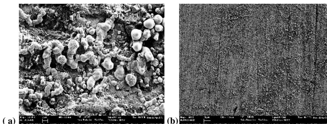
Fig. 1: SEM image of the surface of low alloy steel after immersion for 4 h in 1 M  $H_3PO_4$  at 30°C in absence and presence of inhibitor *Calotropis procera*
