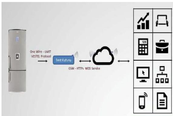
Figure 6. One Wire Connection
