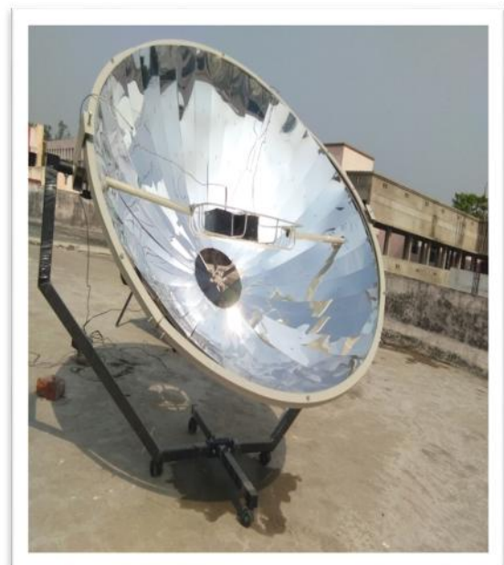
Figure1: Experimental set-up of the parabolic solar cooker.
