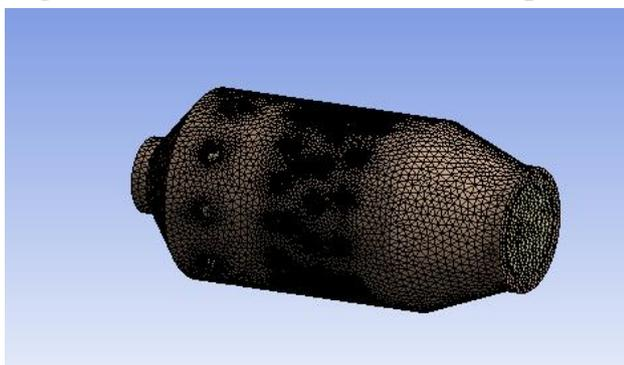
Fig. 4.2: - Tube-Annular Combustor (Meshed)
