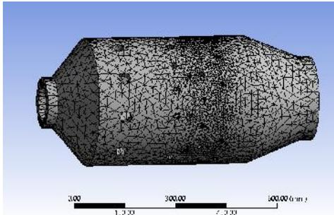
**Fig. 4.8:- Tube-Annular Combustor (Meshed)**
