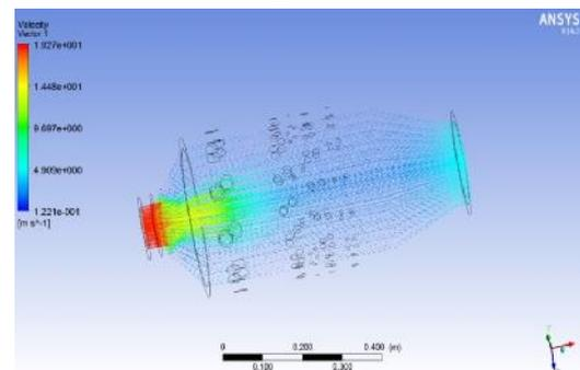
Fig. 4.6 : - Tube-Annular Combustor (Velocity)
