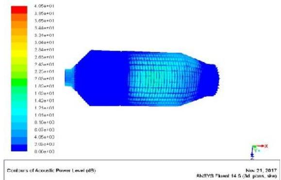
Fig 4.4: - Tube-Annular Combustor (Acoustic power level)
