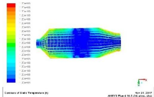
Fig. 4.5 : - Tube-Annular Combustor (Temperature)
