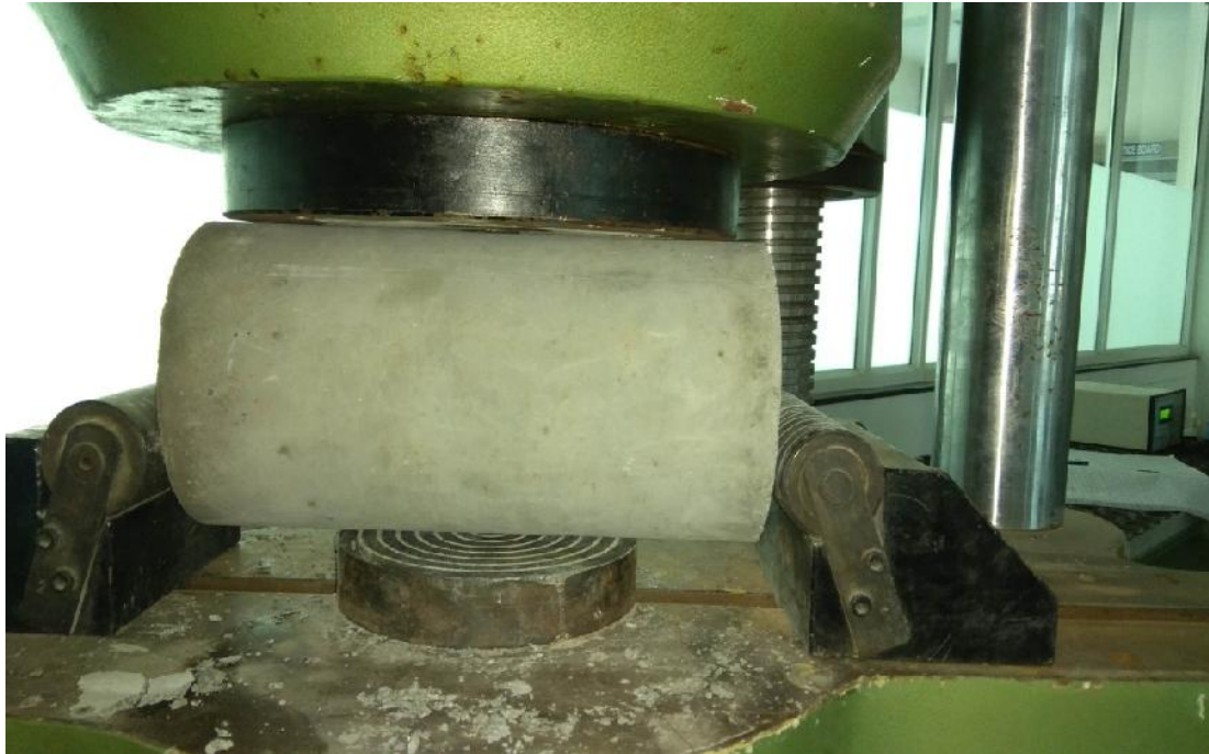
Figure 4: Split tensile test
