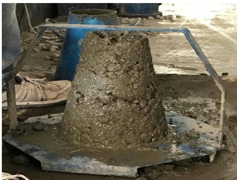
Figure 3: Slump cone test
