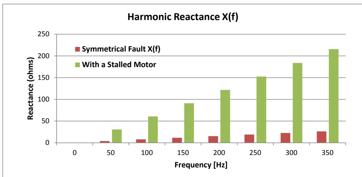
**Figure 9: Comparison of Harmonic Reactance X(f) of Symmetrical fault with a Stalled motor**
