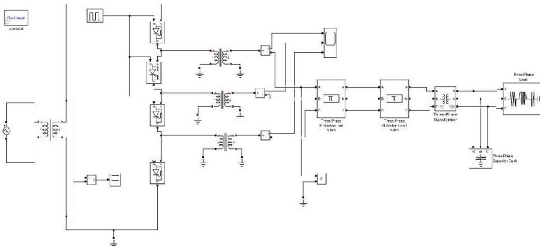
**Figure 10: Simulation of de-energized distribution feeder with a Capacitor bank in downstream.**
