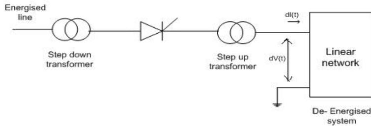
**Figure 2: Downstream de-energized lines a linear network**
