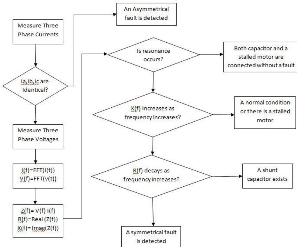
Figure16: Flowchart for overall logic of symmetrical fault detection
