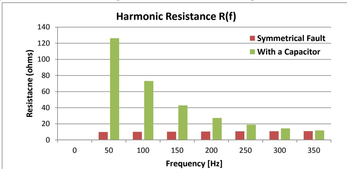
**Figure 11: Comparison of Harmonic Resistance R(f) in No-Fault and Symmetrical fault conditions**
