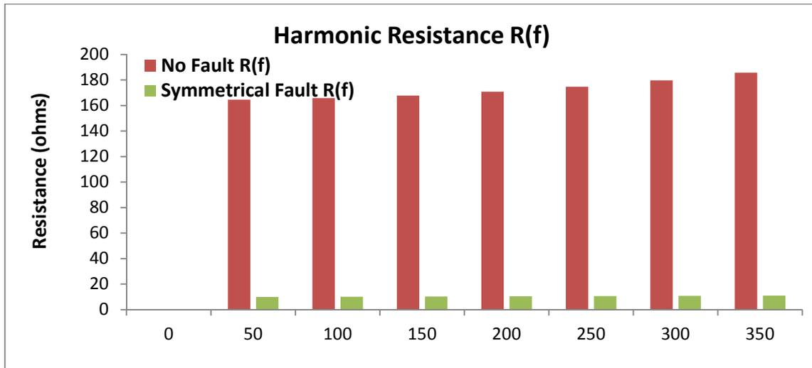
**Figure 6: Comparison of Harmonic Resistance R(f) in No-Fault and Symmetrical fault conditions**
