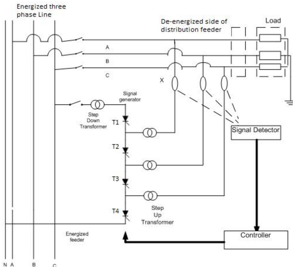
Figure 1: Proposed scheme for symmetrical faults detection.
