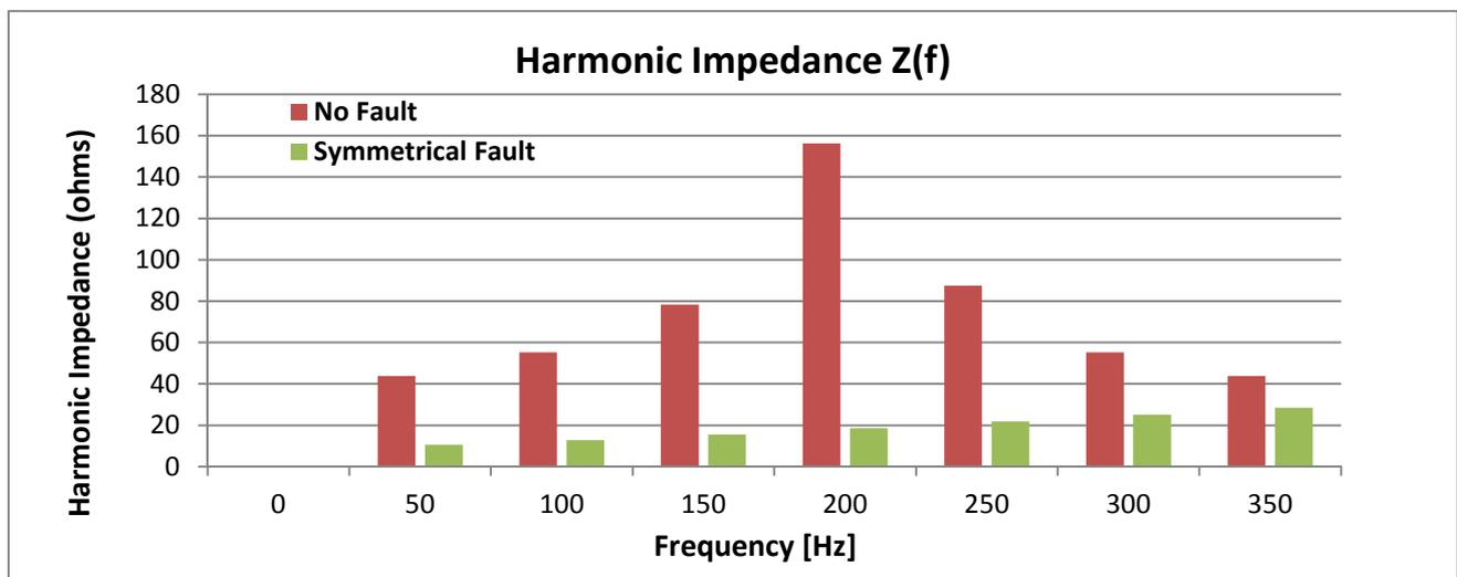
**Figure 13: comparison of Harmonic impedance characteristics when a 2.5 MVA capacitor and a 5000hp motor are connected in downstream.**
