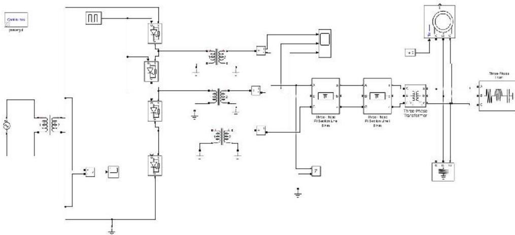
**Figure 8: Simulation of de-energized distribution feeder with a Stalled Motor**
