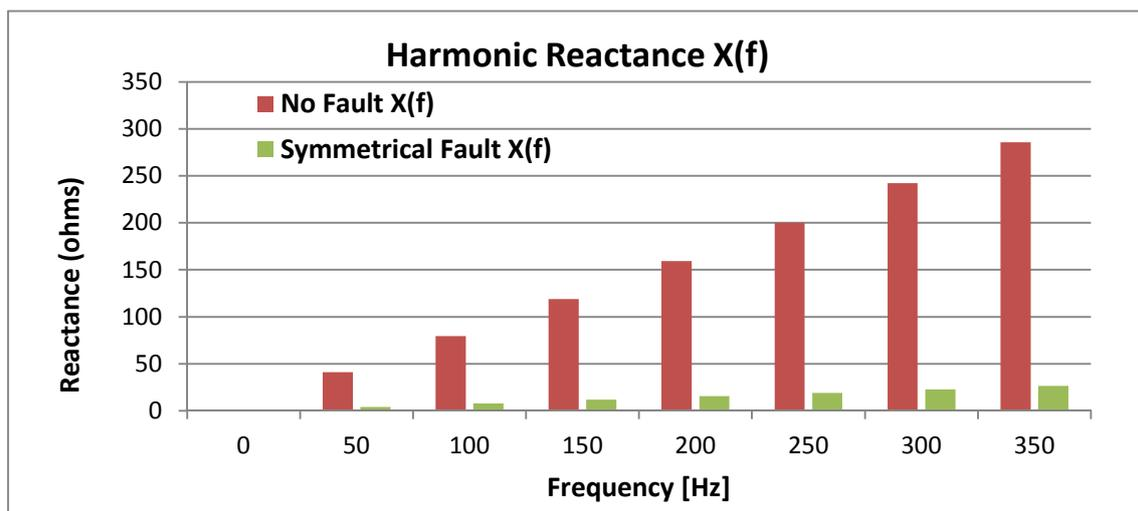
**Figure 7: Comparison of Harmonic Reactance X(f) in No-Fault and Symmetrical fault conditions**
