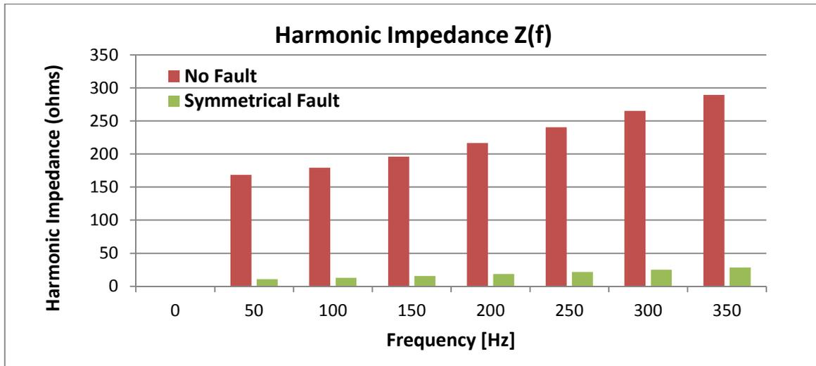
Figure 14: comparison of Harmonic impedance characteristics when a 0.25 MVA capacitor and a 5000hp motor are connected in downstream.
