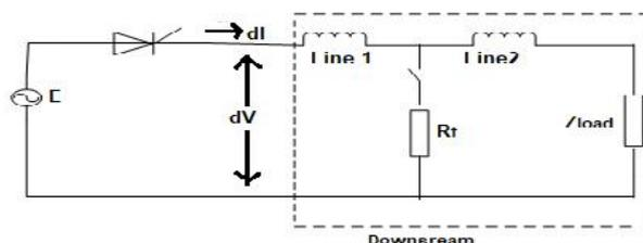
**Figure 3: Equivalent circuit of the proposed idea**
