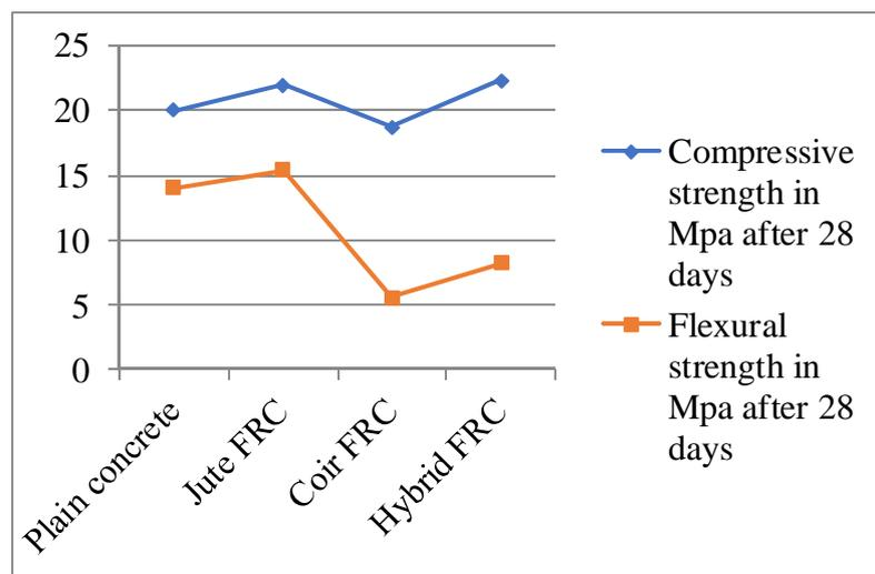
Fig. 7 Obtained Strength Characteristic
