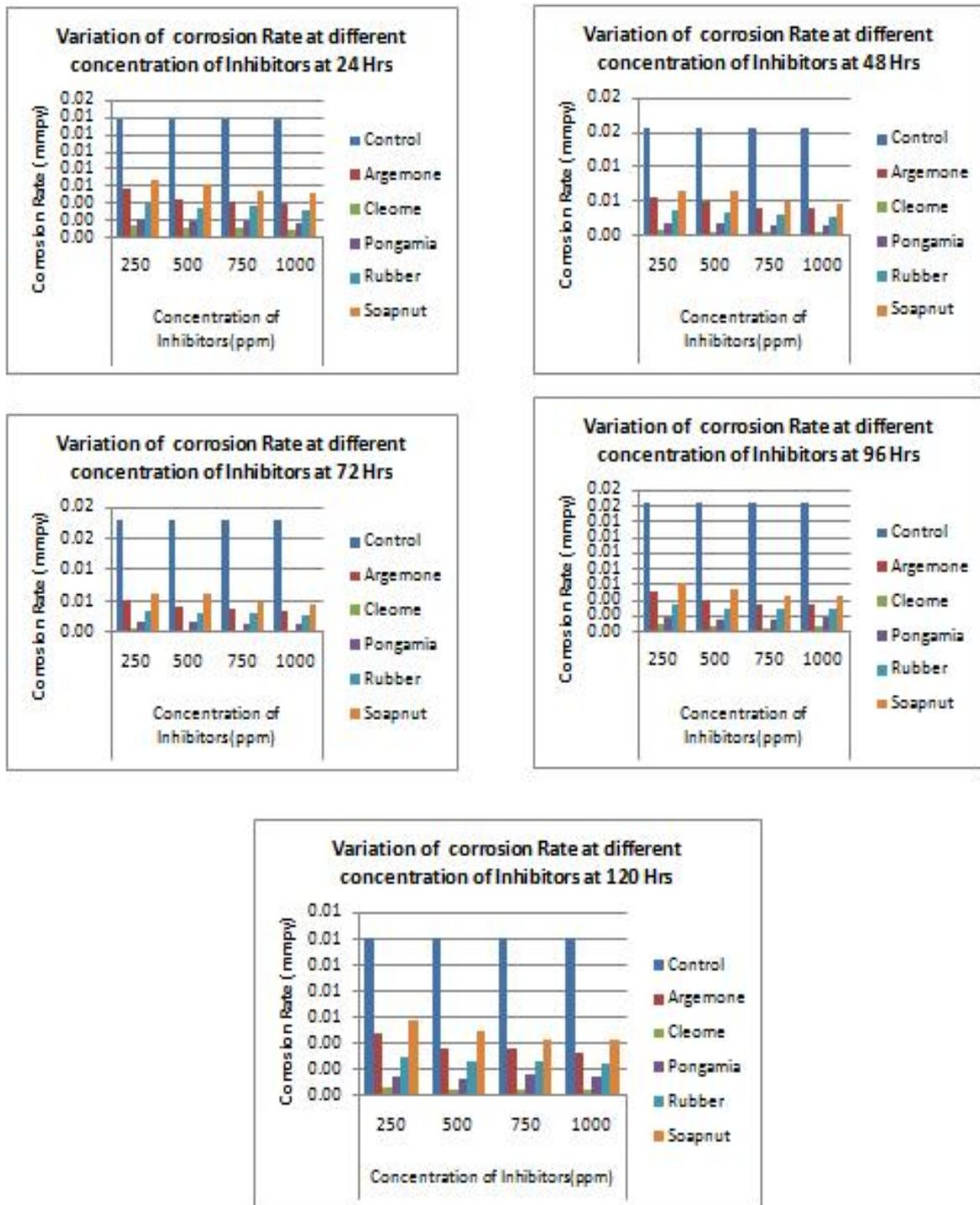
Figure 1 : Variation of corrosion rate at different concentration of Inhibitors at different time duration
