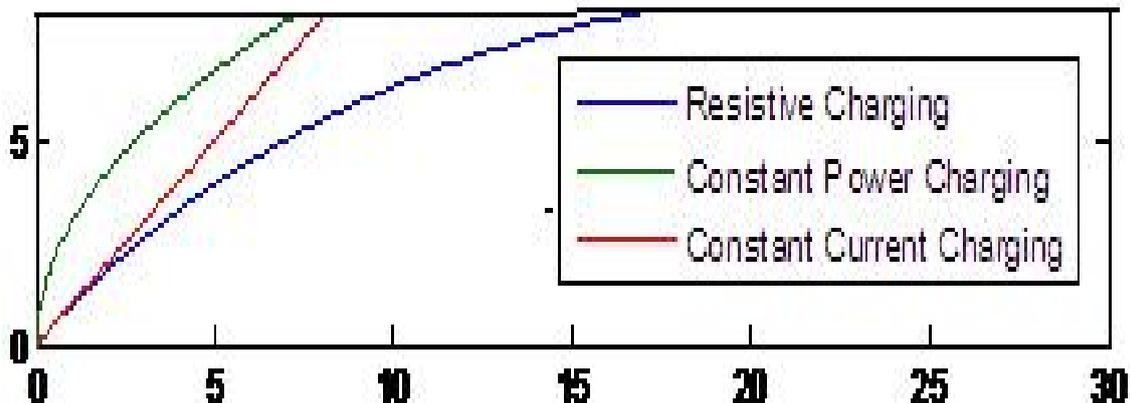
Fig.3 Comparison of Characteristics the Different Charging Scheme.
