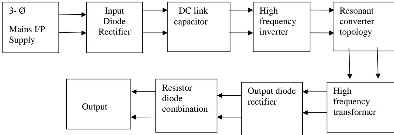
Fig. 4 Blocks of 30 kV, 3 kJ Capacitor charging power supply.
