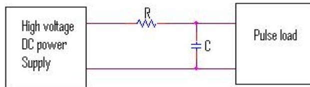
Fig. 1 Schematic diagram of Resistive Charging
