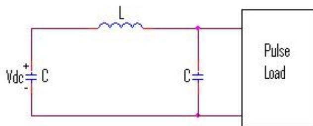
Fig. 2 Schematic of Resonant charging
