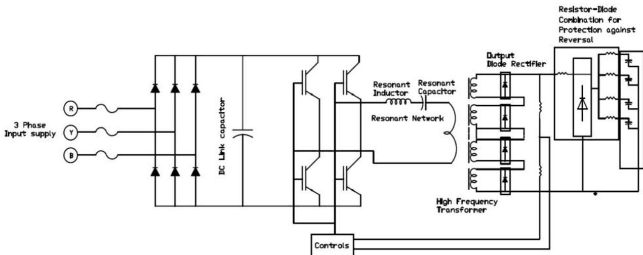
Fig. 5 Schematic diagram of 30 kV, 3 kJ Capacitor charging power supply
