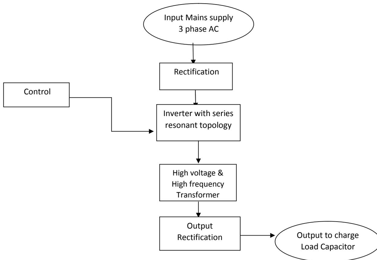
Fig.6 Flow chart of 30 kV, 3 kJ/s Capacitor charging power supply
