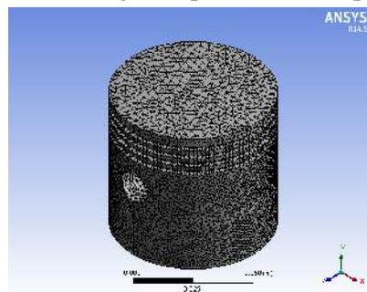
Fig.3 Meshing of a piston
