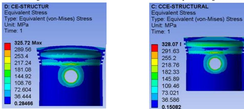
Fig. 6 Stress in conventional and coated piston engine
