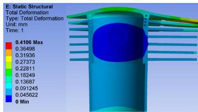
Fig.8 Deformation in copper coated piston and liner assembly
