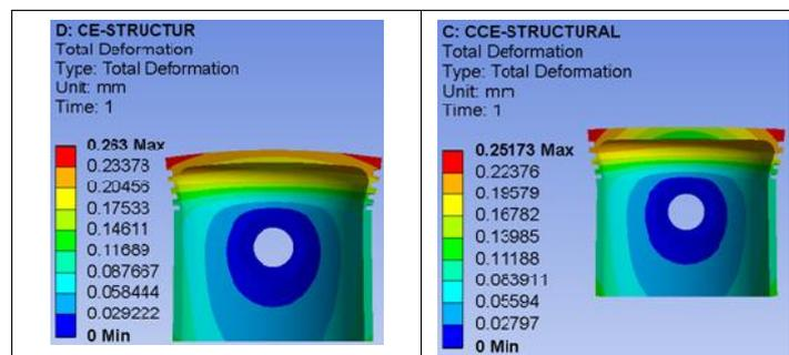
Fig. 5 Deformation in conventional and coated piston engine
