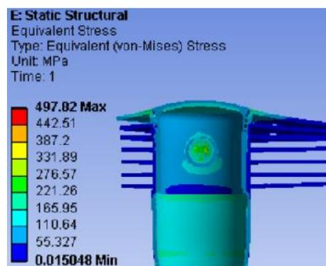
Fig. 9 Von-misses stress in copper coated piston-liner assembly
