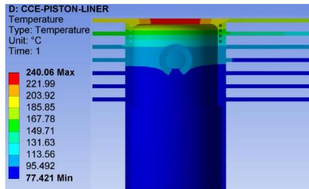
Fig.7 Nodal temperature in copper coated piston and liner assembly
