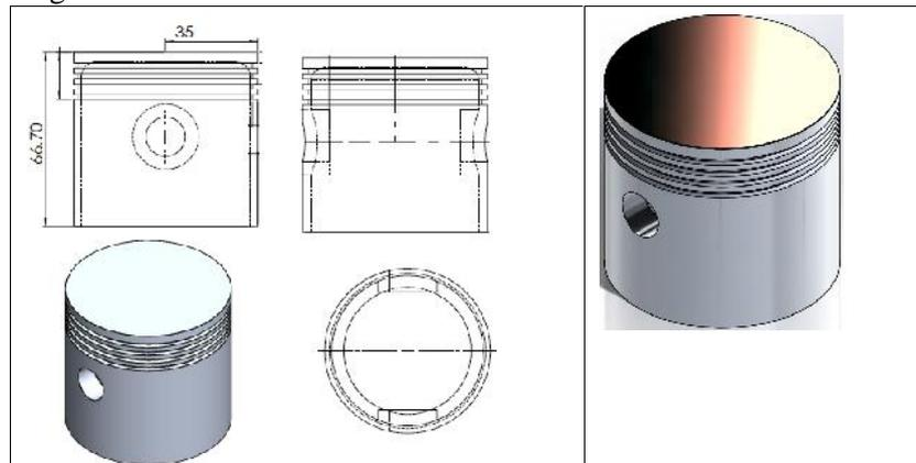
Fig.2 Solid modeling of a piston with copper coating
