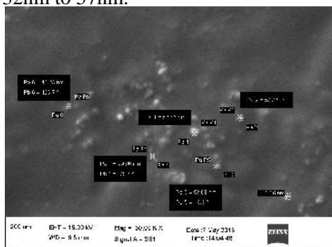
Fig .1 SEM image of silver nanoparticles formed using *Celastrus Paniculatus* leaf extract
