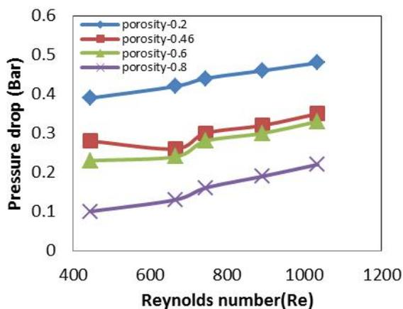
Fig 6. Variation of pressure drop against Reynolds number core diameter 43.5 mm
