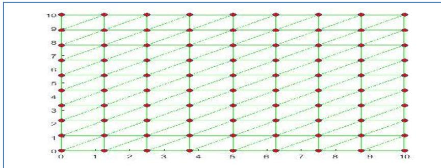
Fig. 3. Typical Mesh for the solution of porous medium problem
