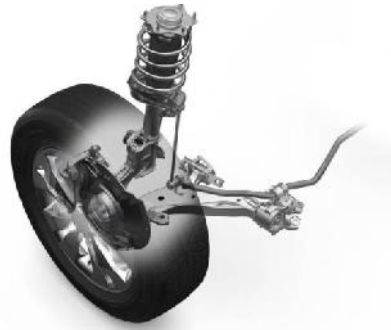
Figure:2 Independent Suspension System:
