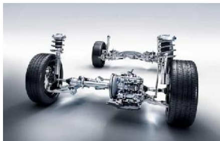
Figure:3 Semi-Independent Suspension System
