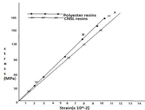
Figure 11: Graph of tensile strength against strain of polyester and CNSL resins reinforced with glass fibers
