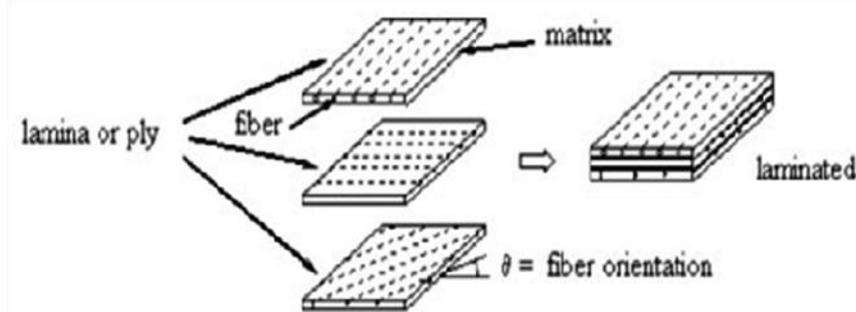
**Figure 6: Laminated (Multilayer) fibers composites**
