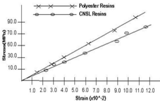
Figure 10: Graph of compressive stress against strain of polyester and CNSL resins reinforced with glass fibres
