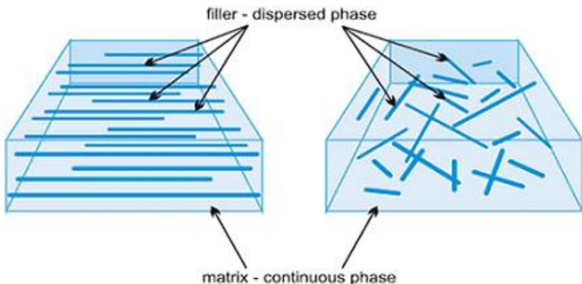
**Figure1: Matrix and dispersed phase of composites**
