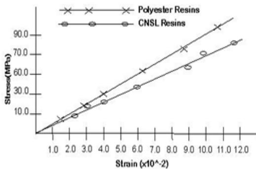
Figure 8: Graph of compressive stress against strain of unreinforced polyester and CNSL resins
