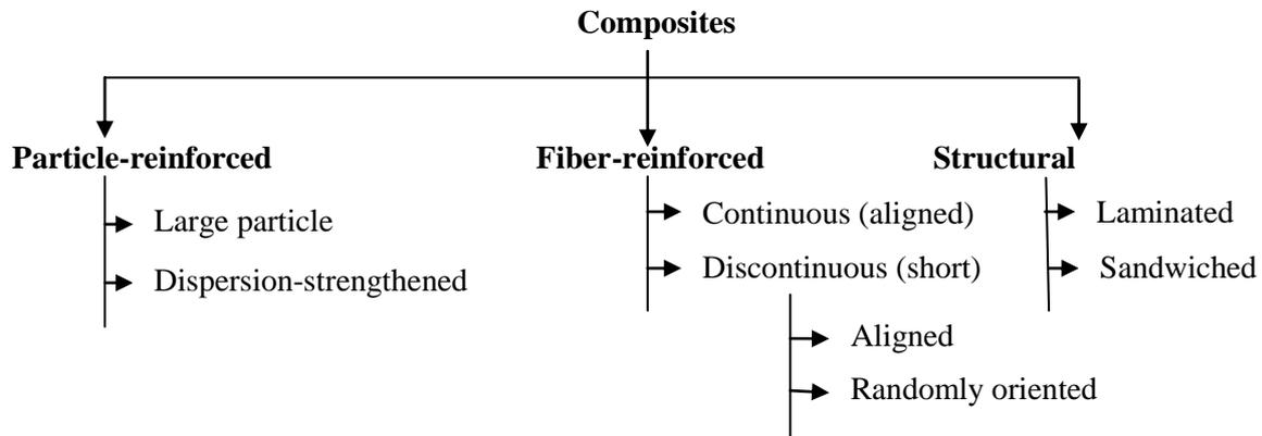
**Figure 2: On the basis of reinforcement**
