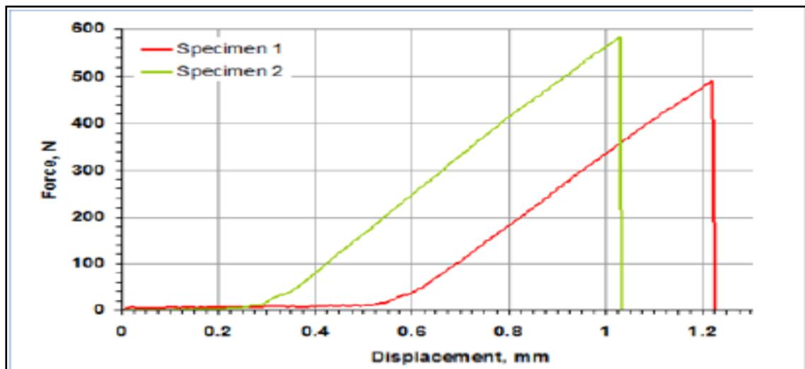
**Figure 12: Shows the force displacement curve for bicomposite with 20% walnut shell particle and 10% coconut fibre [23].**
