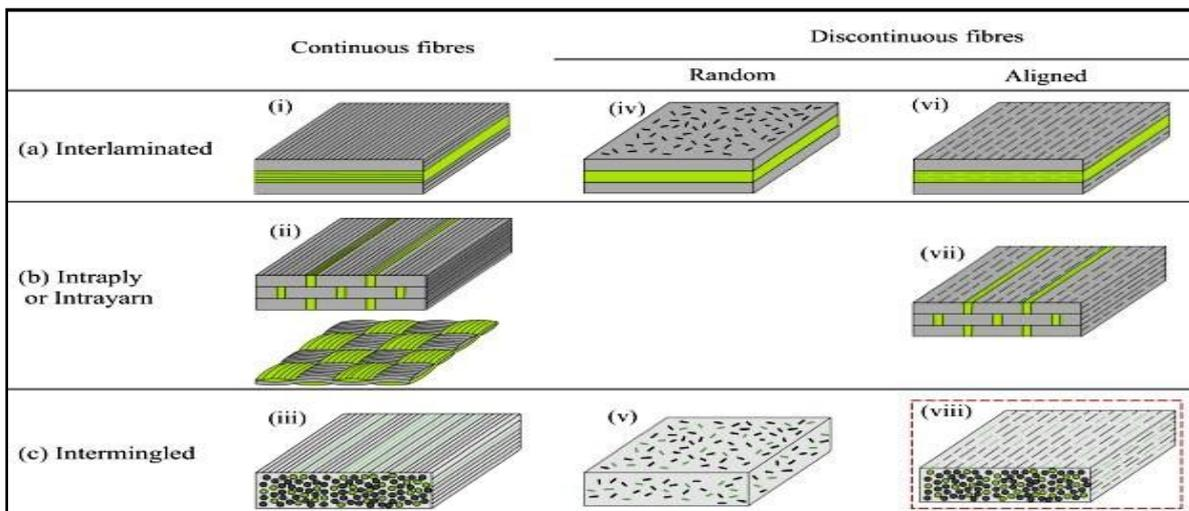
**Figure 5: Continuous and discontinuous fiber composites**
