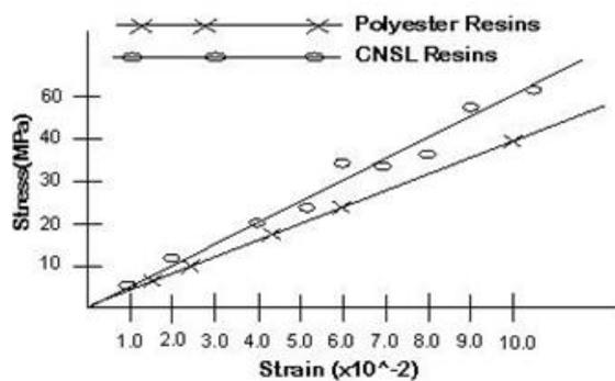
Figure 9: Graph of tensile stress against strain of unreinforced polyester and CNSL resins
