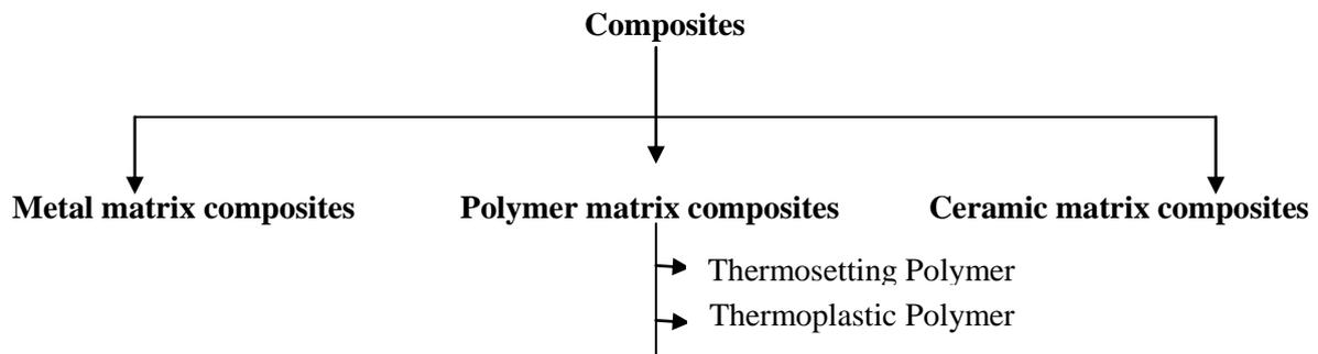
**Figure 3: On the basis of matrix material composites**
