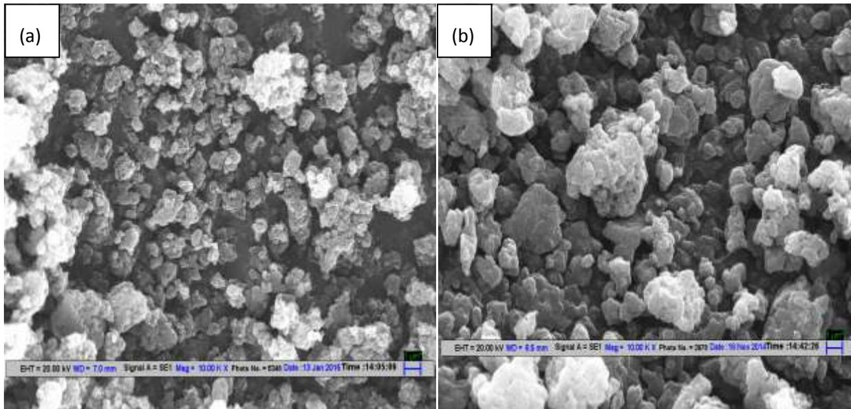
**Figure 1: SEM of (a) PANI (b) PANI/  $\text{CrCl}_3 \cdot 6\text{H}_2\text{O}$  composite ( $\text{CrCl}_{120}$ )**
