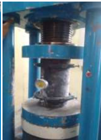
Fig. 4 E for concrete
