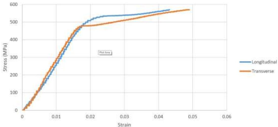
Figure 1: Stress-strain behavior of Inconel 625 in uni axial compression
