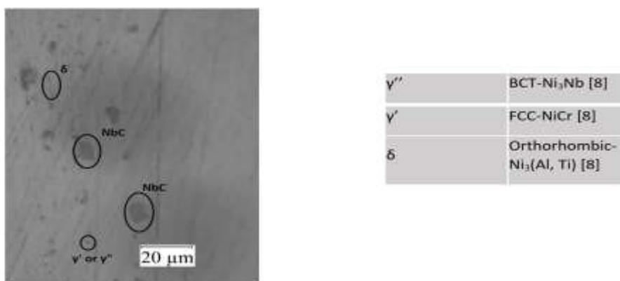
Figure 2: Identification of precipitates in the optical micrograph of Inconel 625
