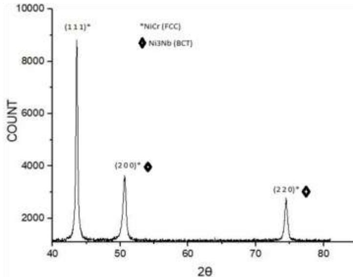
Figure 4: X-ray diffraction patterns for Inconel 625
