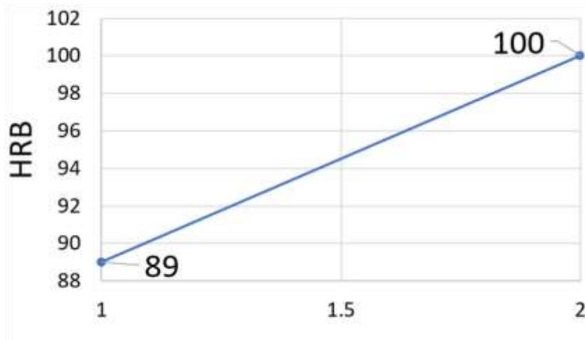
Figure 3: Hardness value in longitudinal (bottom left) and in transverse (top right) of Inconel 625
