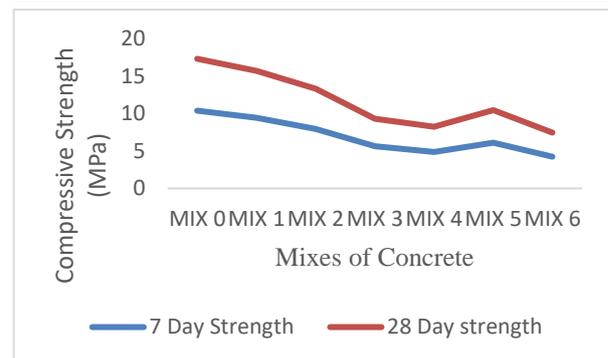
**Fig. 3.** Compressive Strength of Concrete Cubes After 7 Days And 28 Days.
