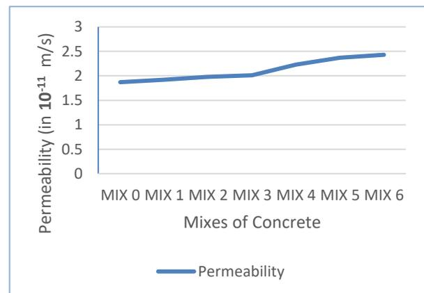
**Fig. 4.** Permeability of Concrete Cylinders After 28 Days.
