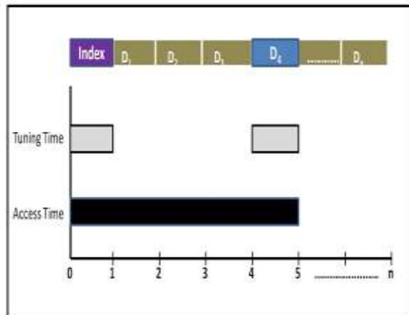
Fig: 6 Indexed data transmission details
